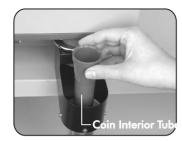
Insert a preformed paper coin tube into the Coin Interior Tube. Slide the paper coin tube down until the bottom contacts the Hook Holder.
