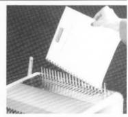
Insert punched sheets face down into the open comb. Push the handle back to bind.
