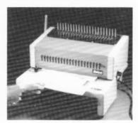
Set adjustments-paper guide, punching die pattern, punching depth selector, and comb opening mechanism. Insert sheets flush against rear stop and paper guide and activate punch with foot pedal.
