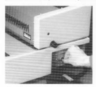
Turn power on. The on/off switch is located on the right side of the machine. Position the foot pedal for operation.
