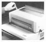
Place binding comb behind metal teeth and spread open by pulling the handle forward.
