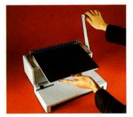
4 Place the punched sheets face down in the binding comb and return the handle to it's original vertical (neutral) position.
