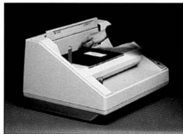
Second, add covers and strip and align document on bind surface.
