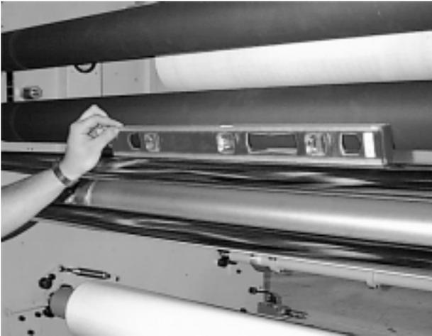
Figure 2-8: Leveling Side to Side
