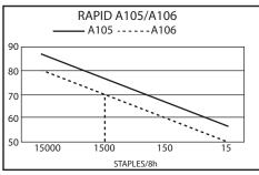
Equivalent noise level dB(A) at maximum capacity and power.
