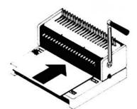
Pull the handle down for punching. Return the handle to its upright position to remove the paper.
