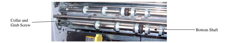
The bottom shaft can not be removed from the machine but can be slid across to allow components to be removed and repositioned.
