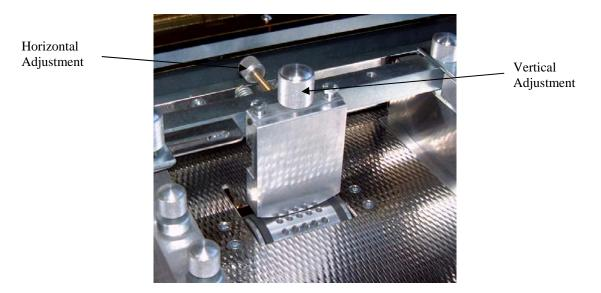
The feed gate is set to allow only one document past at a time. This is achieved by altering the gap and position of the bottom edge of the gate to the rotating cylinder. There are two thumbscrew adjustments. One on top, to allow the vertical movement of the gate, and one under the top cover, to allow horizontal movement. Adjustment of the gate carried out along with adjustment of the choke.
