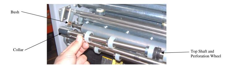
The top shaft must be in its raised position to be removed. It is removed by undoing the grub screw in the collar on the left hand end and sliding the collar to the right and out of the bush, allowing the end of the shaft to come towards you. It can then be removed from its location on the right hand side. The components on the shaft can then be loosened, slide off and repositioned in the desired order.
