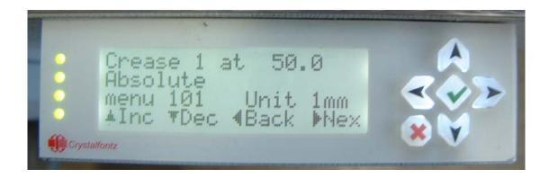
Line 1 shows which crease line is being programmed and what its current value is in mm.
