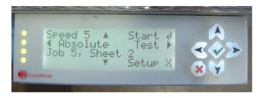
The Operator Run Screen will be displayed under normal run conditions.
