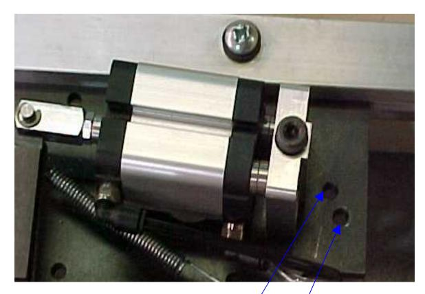
Mount the air cylinders in the top inside holes for C-size blade configuration.
