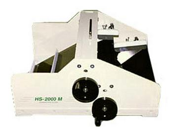
The HS-2000 M is a manual business card making machine that works by inserting letter sized paper with cards printed in a 10 up format. The business cards get cut by hand cranking them through. It is ideal for use in low end situations where you run at 10 up. This slitter will produce standard size 2" x 3-1/2" cards and remove the trim.
