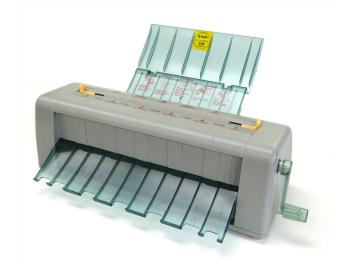
The BCS 1000M business card cutter makes it easy to produce business cards whenever you need them. It is a manual machine with self sharpening blades to always guarantee a clean precise cut. The BCS 1000M Business Card Slitter works by cutting a letter size  $(8\ 1/2" \times 11")$  sheet into two strips and then those two strips into 10 business cards.
