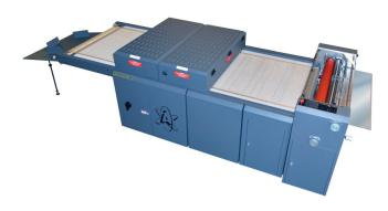
The Spectra-Coat 40" UV Coater is available as a hand-fed unit or with an air feeder. A deep-pile outfeed stacker is also available. It runs up to one-quarter inch thick substrates, with an option of running up to 1 inch thick substrates.
